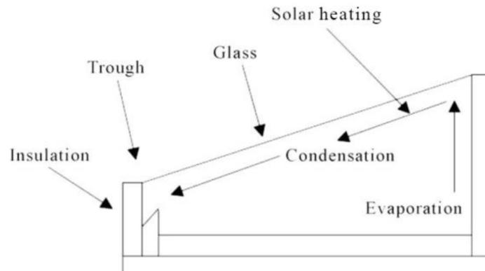
Figure 1.1: A simple schematic of a single basin solar still. Source: Pednekar *et al.* (2018)
