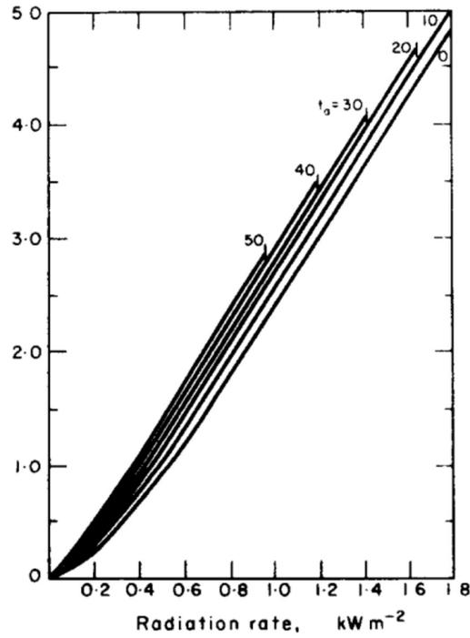
Figure 1.4: Ideal production rate as a function of radiation rate and ambient temperature. Source: Cooper (1973)
