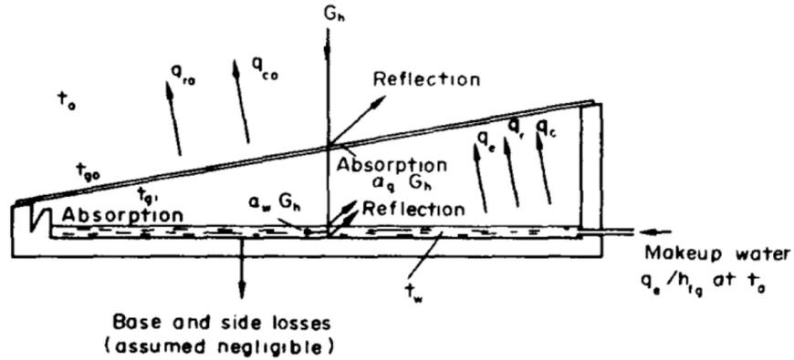
Figure 1.3: Steady state heat flows for a single-effect solar still. Source: Cooper (1973)
