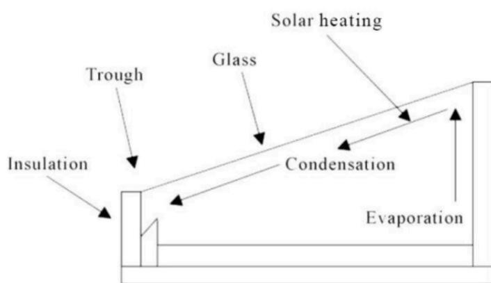
Figure 1: A simple schematic of a single basin solar still [2].
