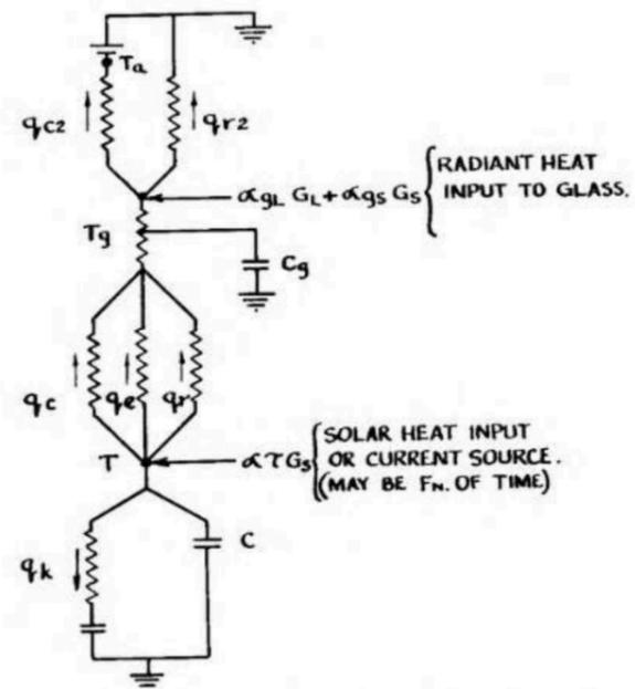
Figure 2: A thermal of a single basin solar still [3].
